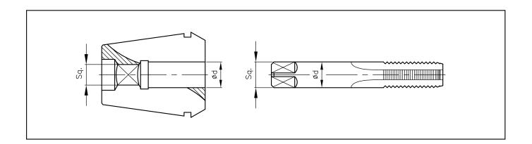
Since there exists number of CNC turning and machining centres equipped with rigid tapping features we developed collet type RDTC & RDGTC.
