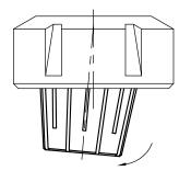
RELEASE: By unscrewing the clamping nut from the collet holder the collet is pulled automatically by means of the eccentric ring in the nut.
