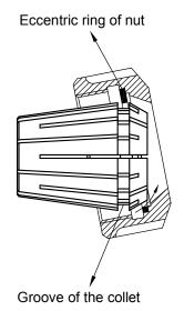
INSERTION: Introduce collet into the clamping nut at an angle as shown in the sketch and turn the nut till it snaps into the groove of the collet.
